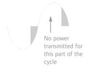
A trailing edge dimmer 'chops' the waveform and only transmits power for the first part of the cycle
